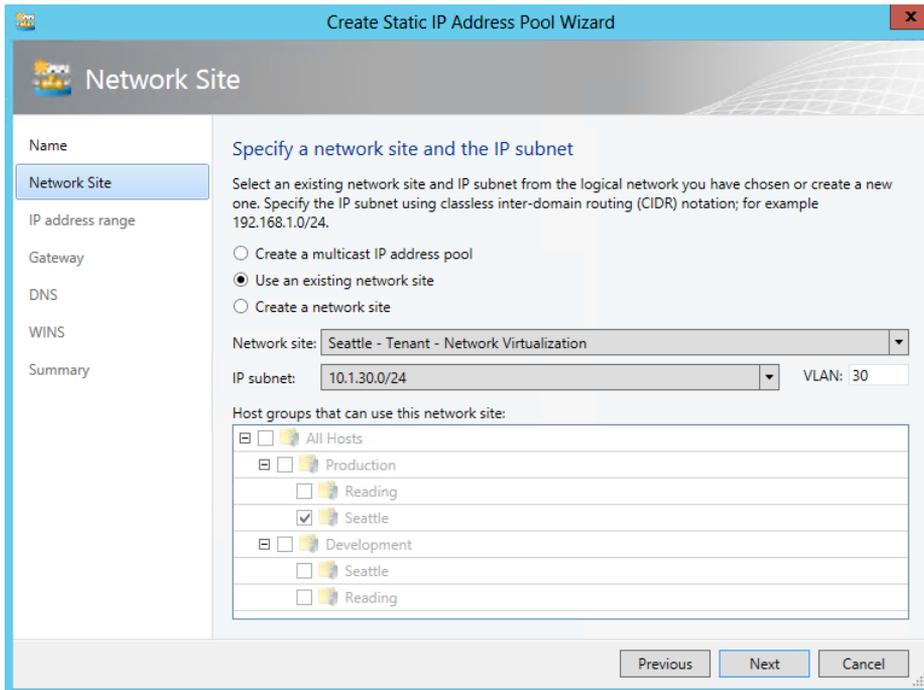
**FIGURE 2-21** Defining a provider address IP pool for a network site
