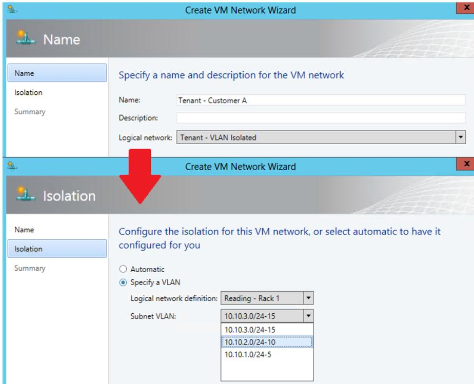
**FIGURE 2-12** Allocating a VLAN (network site) to a VM network
