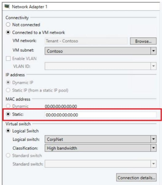
**FIGURE 7-2** Configuring a network adapter to use a MAC address from a MAC address pool
