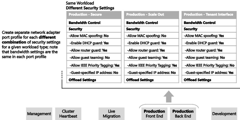
**FIGURE 3-18** Refined solution for workloads with different security settings
