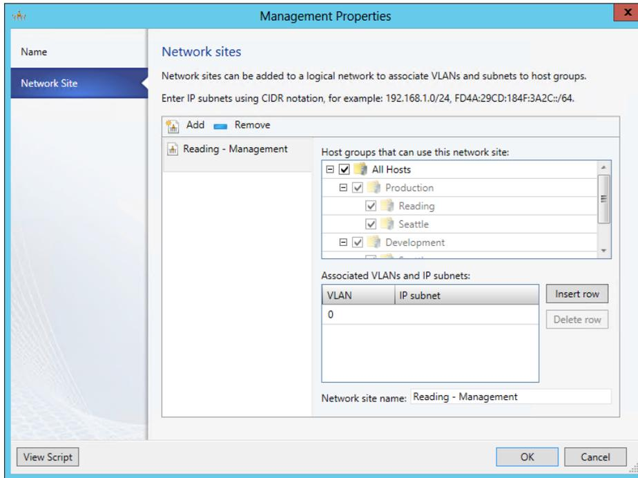
**FIGURE 6-2** Example of an untagged host management logical network
