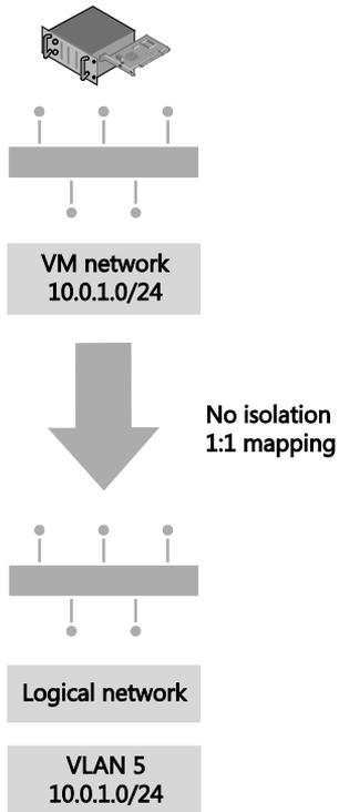
**FIGURE 2-9** VM network direct access to the logical network
