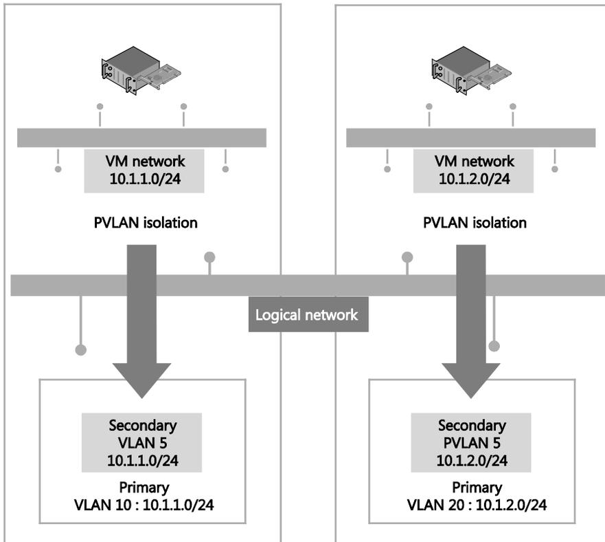
**FIGURE 2-18** Logical network design for PVLAN isolation
