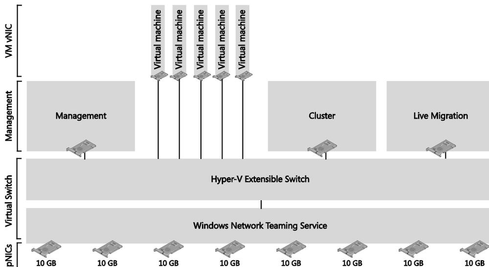
FIGURE 4-7 Fully converged network example
