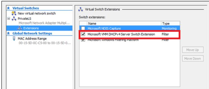
**FIGURE 8-1** A Hyper-V switch with the VMM DHCPv4 Server Switch Extension enabled
