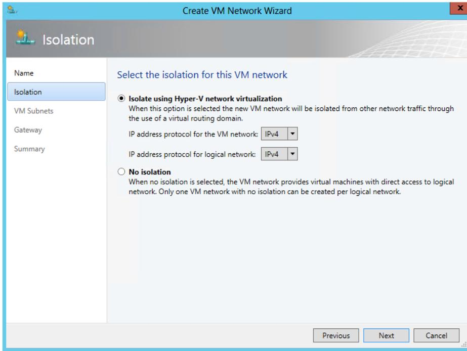
**FIGURE 2-22** VM network isolation using Hyper-V Network Virtualization
