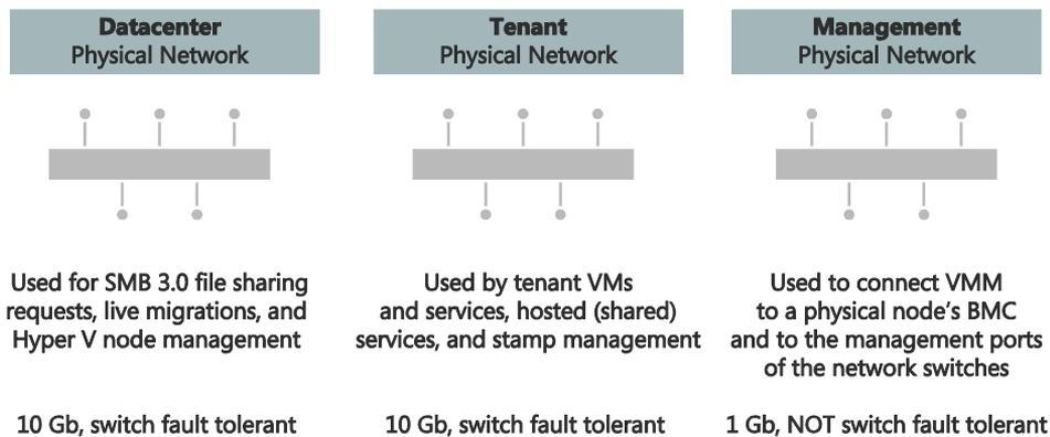
**FIGURE 9-5** The three physical networks present in a CPS rack
