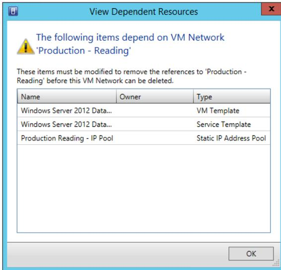
**FIGURE 7-4** Checking for dependent resources prior to VM network deletion
