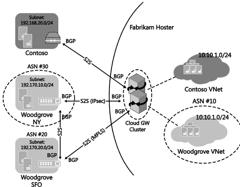
**FIGURE 5-4** Connecting multiple sites of an enterprise to a virtual network
