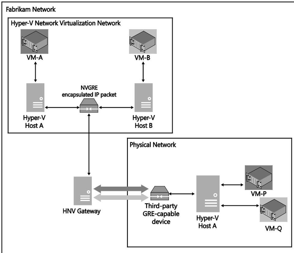
**FIGURE 5-8** Connecting to a legacy network using a GRE tunnel
