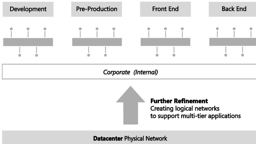
**FIGURE 2-4** Dividing Production into front end and back end logical networks
