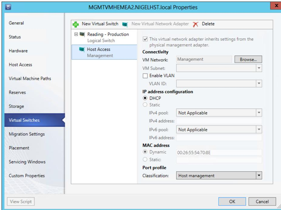
**FIGURE 6-3** Logical switch deployment using untagged host management
