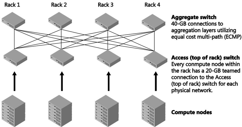
**FIGURE 9-4** Flat network topology used by CPS to connect resources across the stamp
