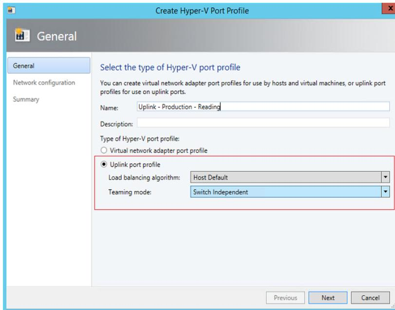
**FIGURE 3-2** Load balancing and teaming mode selections in an uplink port profile
