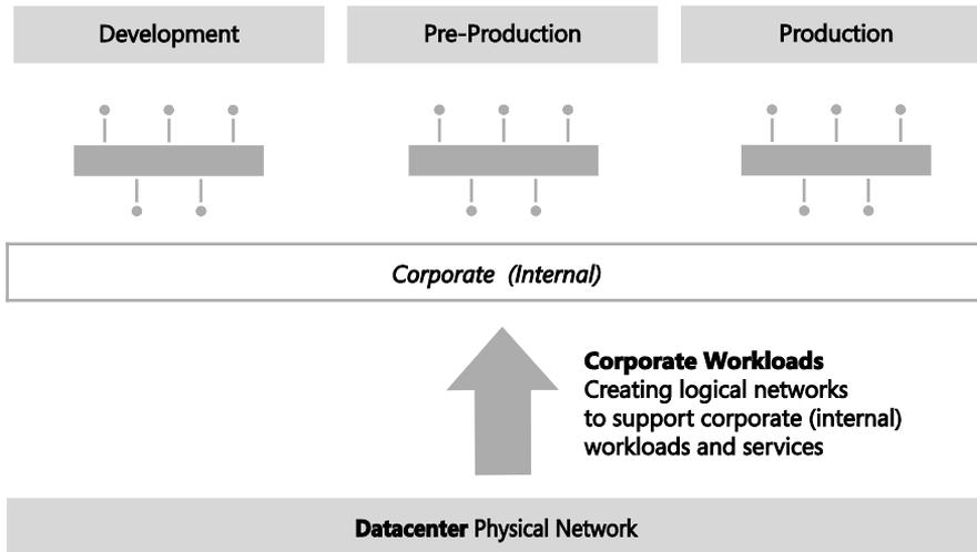
**FIGURE 2-3** Using logical networks to differentiate workloads
