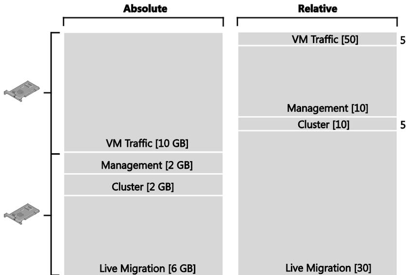
**FIGURE 4-14** Adding minimum bandwidth to relative weights
