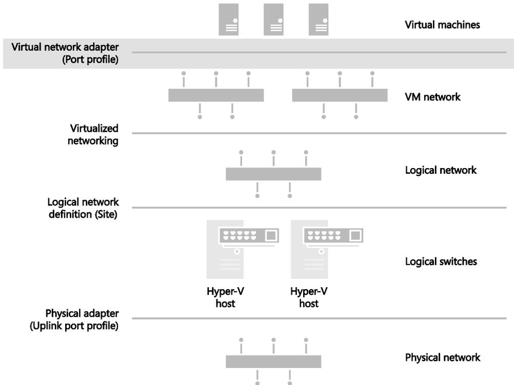
**FIGURE 3-15** Architecture showing network adapter port profiles
