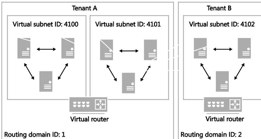
**FIGURE 2-19** Logical network design for isolation using network virtualization
