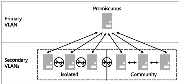
**FIGURE 2-14** The three modes for PVLAN isolation
