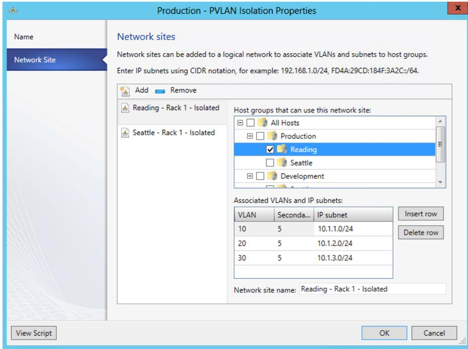
**FIGURE 2-16** Network site configured for PVLAN isolation
