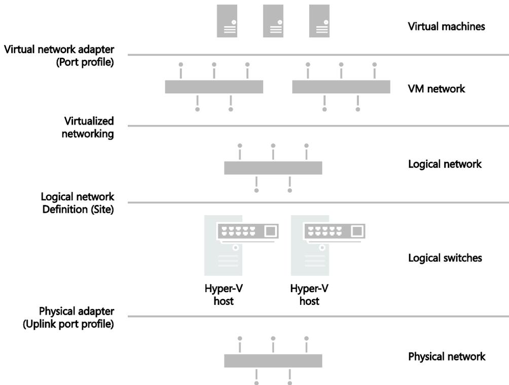
**FIGURE 1-1** Architecture of a virtualized network solution
