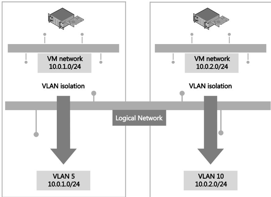
**FIGURE 2-13** Logical network design for VLAN isolation
