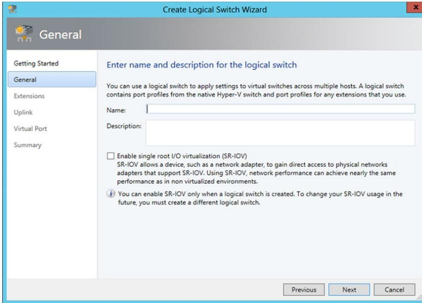
**FIGURE 4-11** Option to enable SR-IOV during the creation of a logical switch
