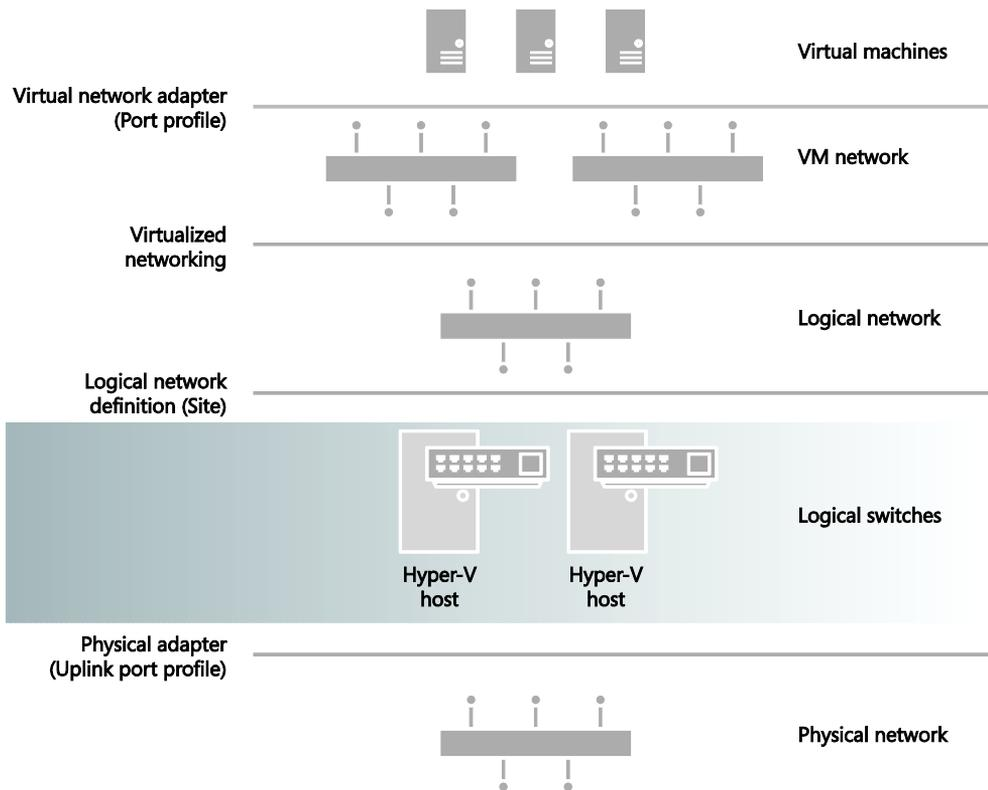
**FIGURE 4-1** Architecture of a virtualized network solution showing how logical switches connect with other features
