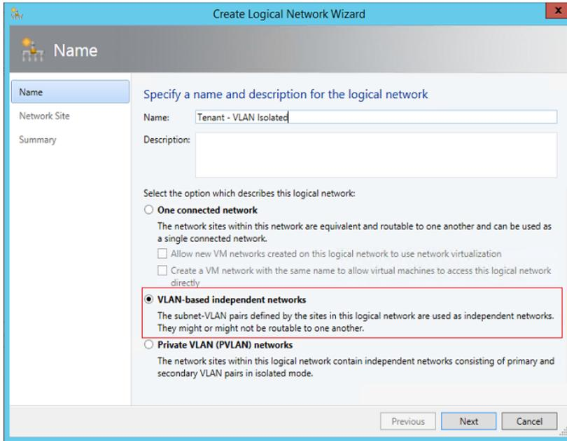
**FIGURE 2-10** Configuring a logical network for VLAN isolation
