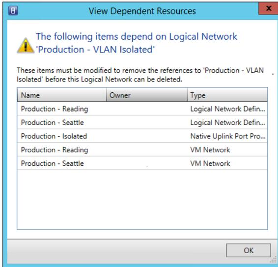
**FIGURE 7-3** Checking for dependent resources prior to logical network deletion
