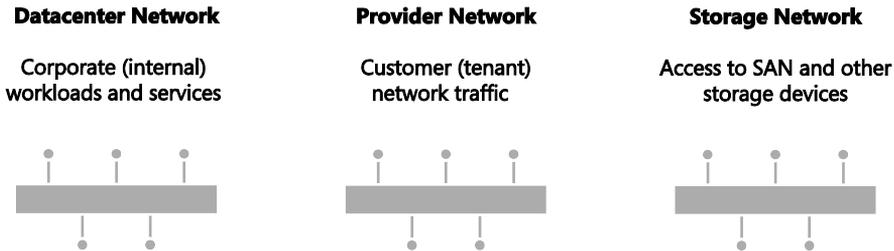
FIGURE 2-1 Physical networks in each Fabrikam datacenter
