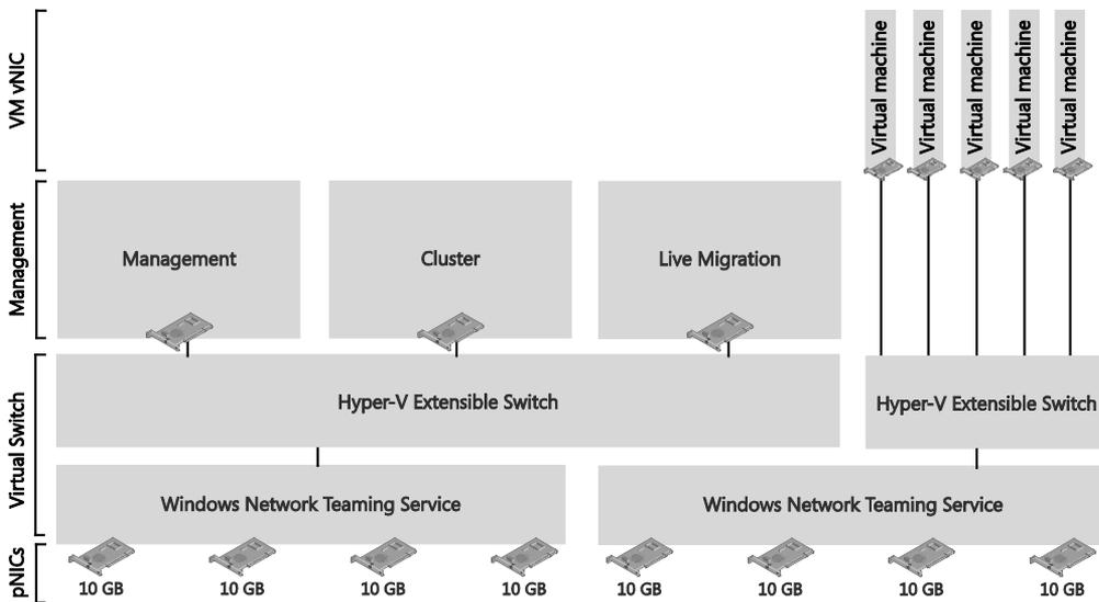
**FIGURE 4-8** Implementing with dual logical switches
