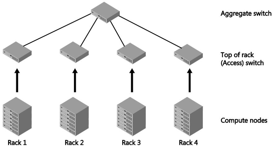
**FIGURE 9-3** Using a hierarchy of switches to connect resources across the stamp
