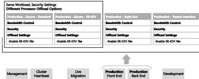
FIGURE 3-19 Adding profiles for network adapters that support offloading
