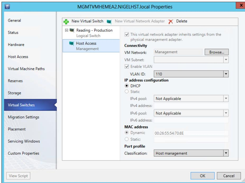
FIGURE 6-5 Logical switch deployment using tagged host management
