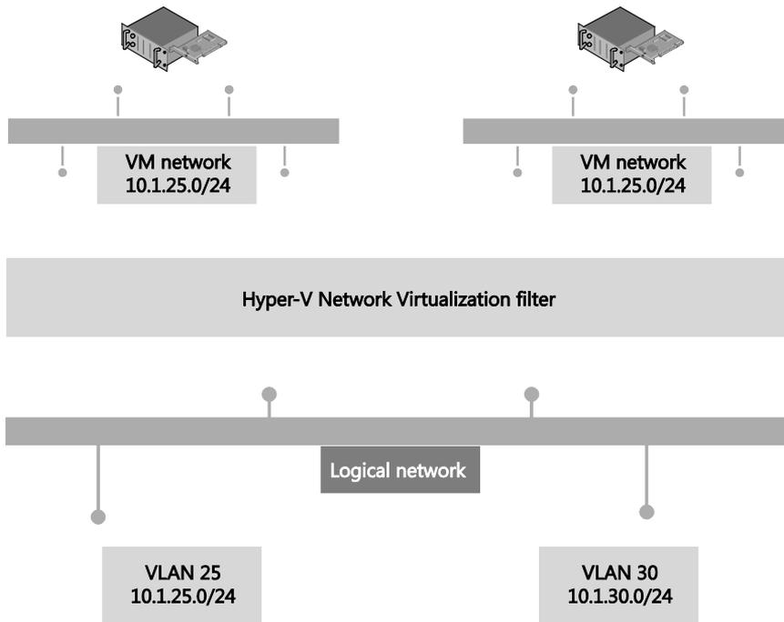
**FIGURE 2-24** Logical network design for network virtualization
