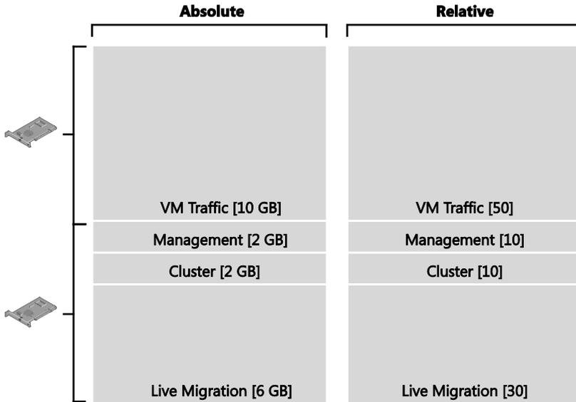
**FIGURE 4-13** Distributing 20 GB of bandwidth using absolute and relative weighting
