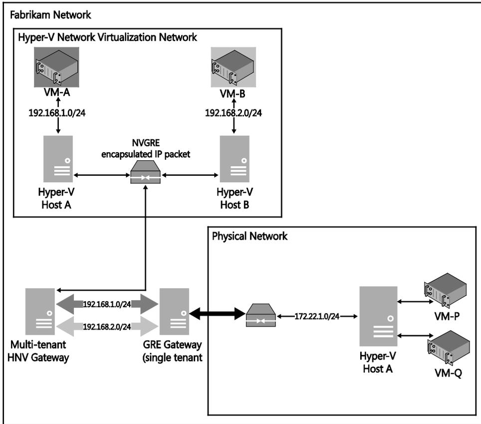
FIGURE 5-6 Integration with non-overlapping IP addresses
