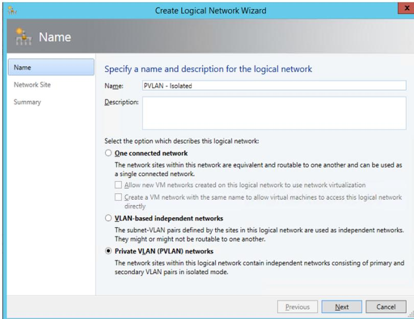
**FIGURE 2-15** Enabling PVLAN isolation
