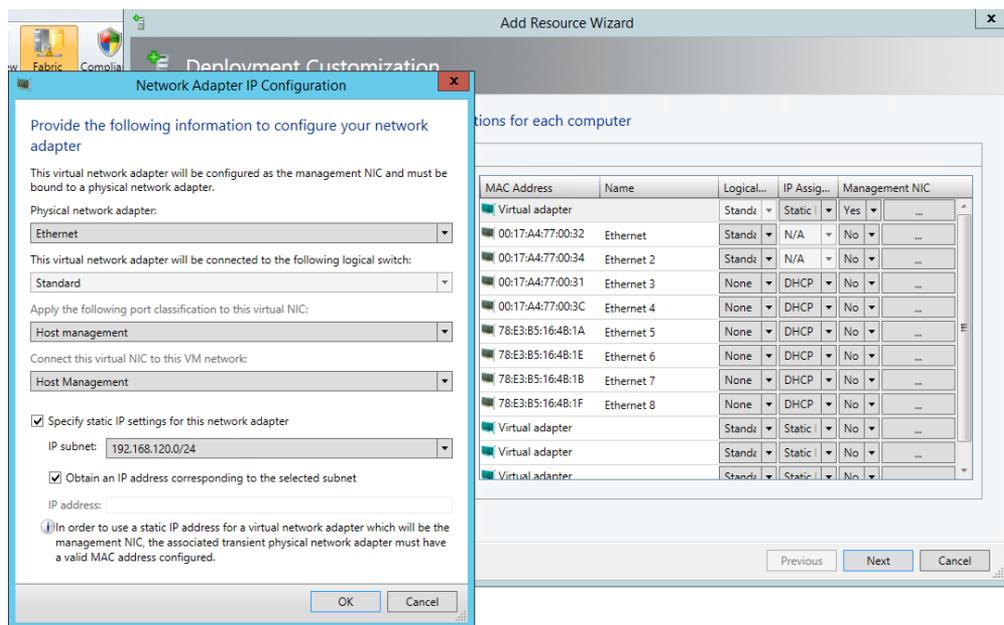
FIGURE 6-7 Bare-metal deployment network configuration
