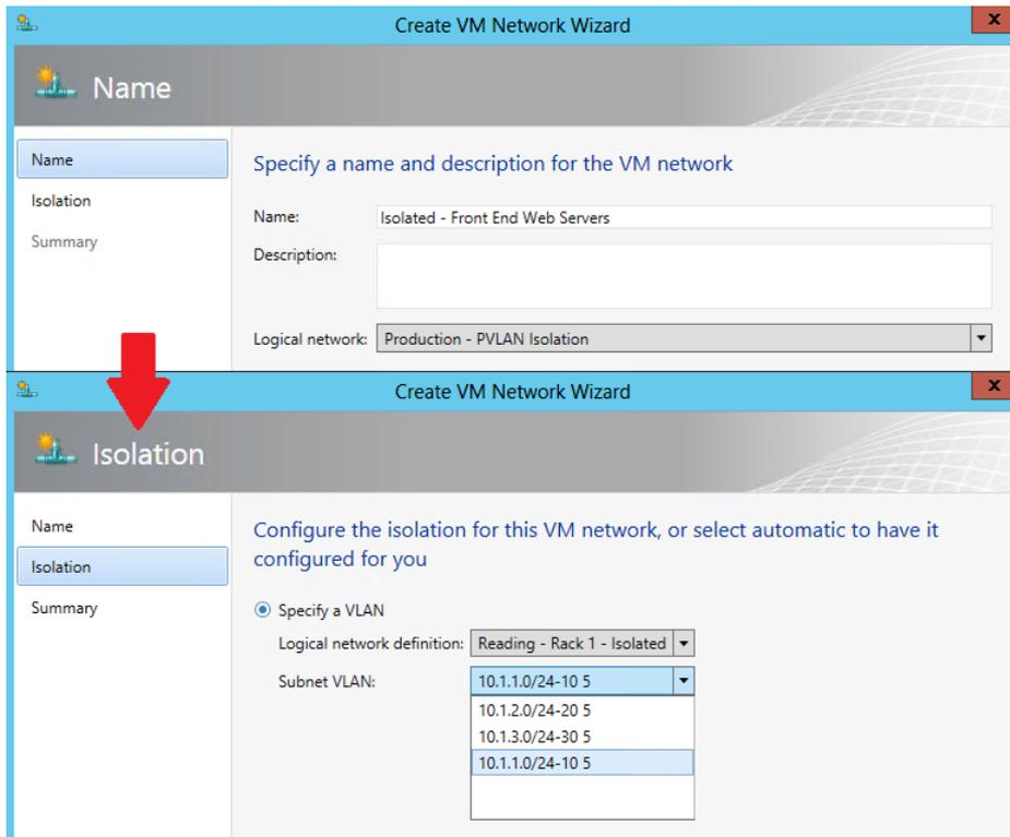
**FIGURE 2-17** Allocating a PVLAN (network site) to a VM network
