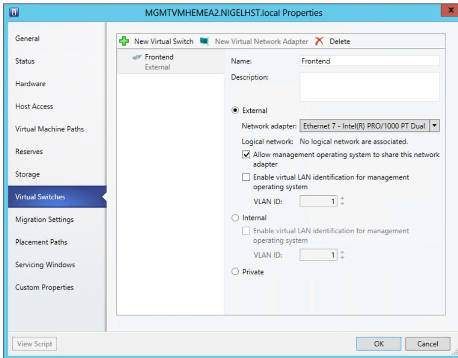
FIGURE 6-8 How a standard Hyper-V switch is represented in VMM
