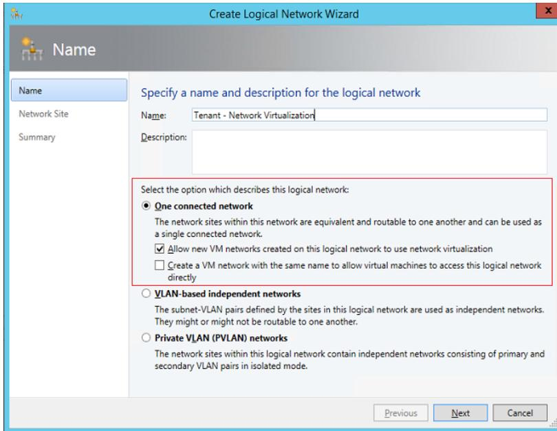
**FIGURE 2-20** Configuring a logical network to support network virtualization
