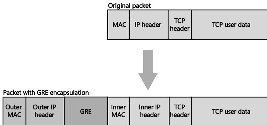
**FIGURE 5-1** Network virtualization using GRE
