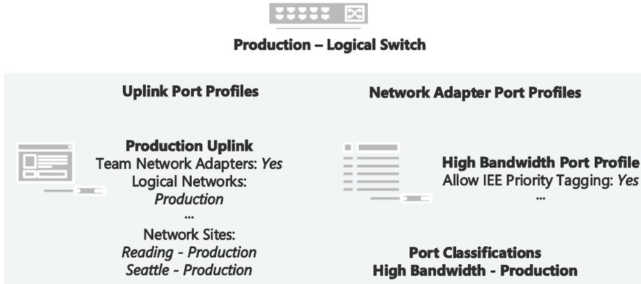
**FIGURE 1-6** Contents of the Production logical switch
