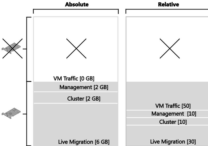
**FIGURE 4-15** Bandwidth weights and minimum reservations with a 10-GB path failure
