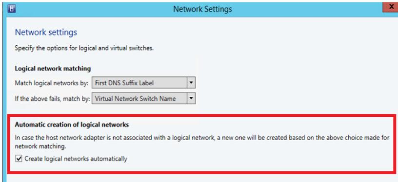
**FIGURE 2-27** Turning off automatic logical network creation
