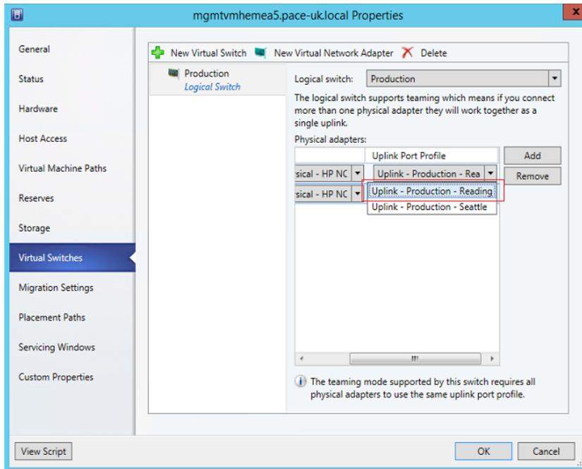
**FIGURE 3-4** Selecting an uplink port profile as part of logical switch deployment
