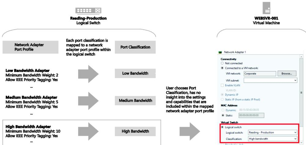
FIGURE 3-16 Applying a network adapter port profile
