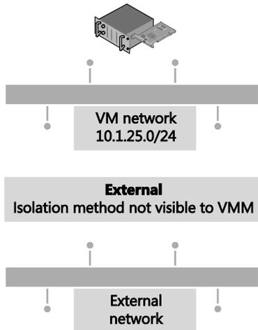
**FIGURE 2-25** Externally defined networks with the isolation method invisible to VMM
