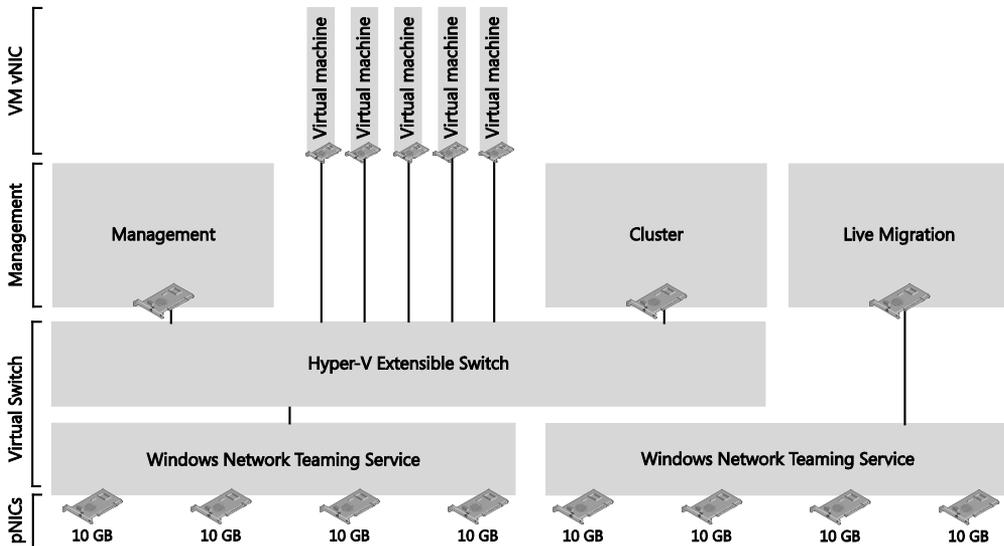
**FIGURE 4-6** Utilizing vNICs to consolidate multiple networks
