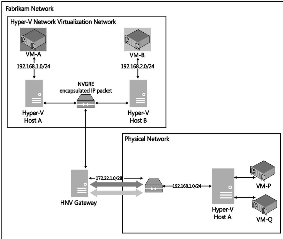
**FIGURE 5-7** Integration with overlapping IP addresses
