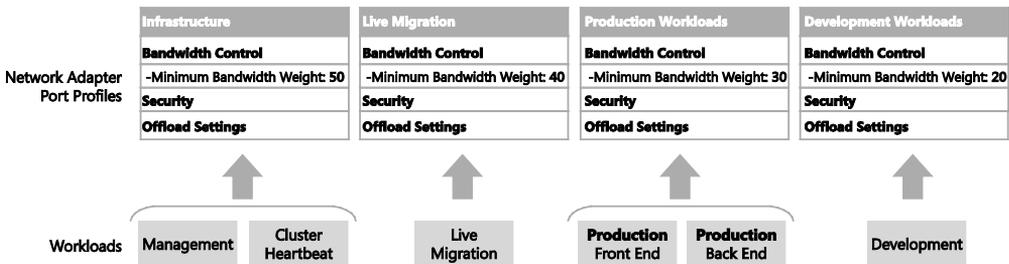
FIGURE 3-17 A network adapter port profile for each prioritized workload
