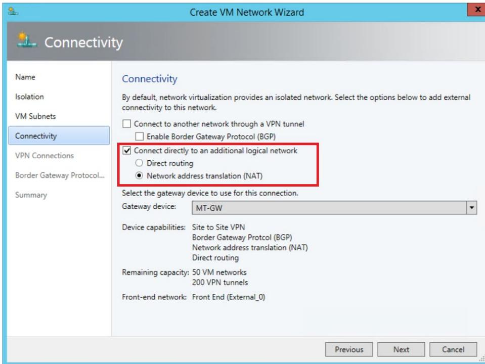
**FIGURE 1-8** Using a gateway to connect a VM network to a public network
