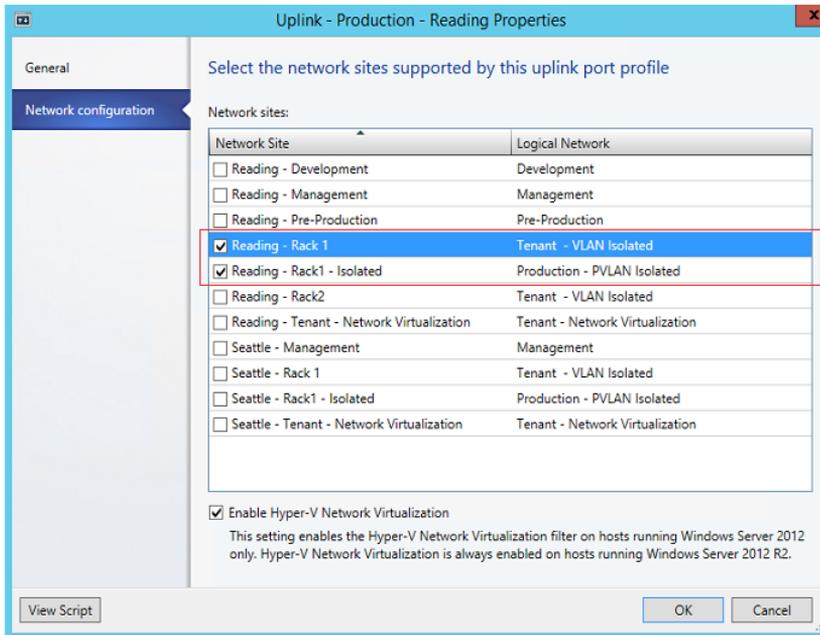
**FIGURE 3-3** Network sites in an uplink port profile
