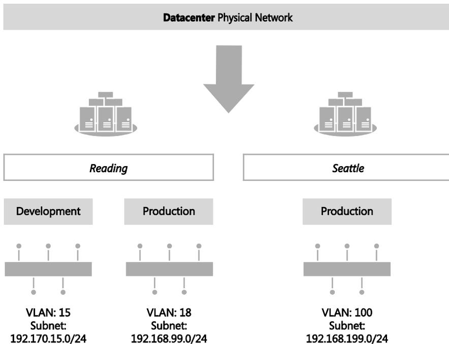
**FIGURE 3-6** Workloads differentiated by VLAN and IP subnet
